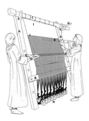
Figure 1. Diagram of Warp Weighted Loom. Based on a drawing from Penelope Walton Rogers *Cloth*and *Clothing*, page 29 (figure 2.21).
