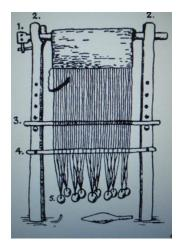
Figure 29. Grace M. Crowfoot drawing of a warp weighted loom. From 'Of the Warp-Weighted Loom', p. 38 (fig. 4). The tool labelled as a 'pin beater' is near the bottom of the left upright of the loom.
